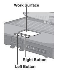
Use the touch pad to move the cursor on the display and perform normal computer operations. For more details, refer to Reference "Touch Pad".
